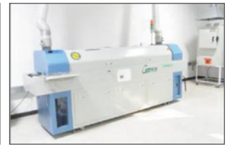
For SMD type products, simulating IR RELOW testing / 高温无铅回流焊机(晋力达)
